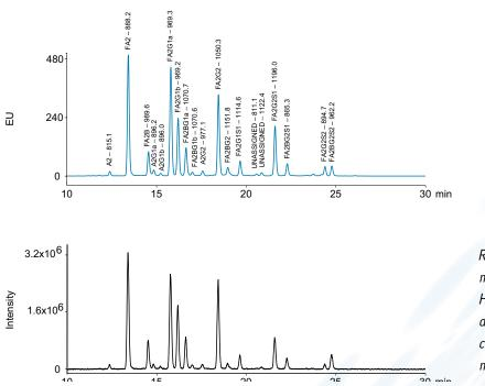
RapiFluor-MS labeled N-glycans monitored using an ACQUITY UPLC H-Class Bio System configured with FLR and ACQUITY QDa mass detection for confirmation of known structures and mass data for unassigned peaks.
