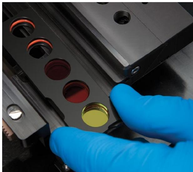
Figure 2. Integrated Filter Slides for GloMax® Discover and Explorer.
